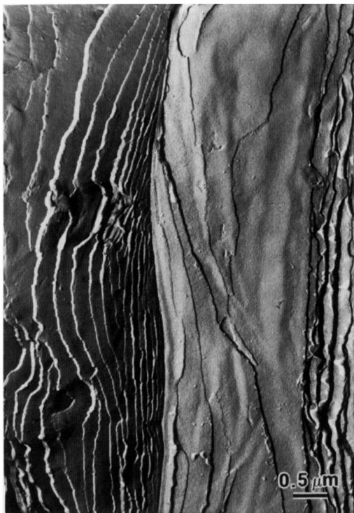
Figure 13 TEM micrograph of a replica from an etched, slow cooled, 'compression moulded' free surface of the C 7 terpolymer
