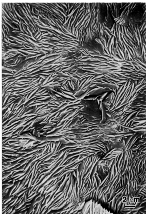
Figure 8 SEM micrograph of an etched cross-sectional fracture surface from a compression moulded, water quenched sample of the C 7 terpolymer
