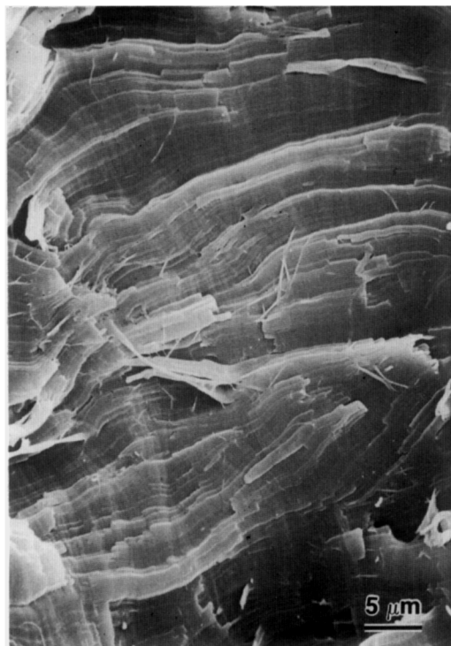
Figure 5 SEM micrograph of a cross-sectional fracture surface (no etching) from a compression moulded, slow cooled sample of the C 7 terpolymer
